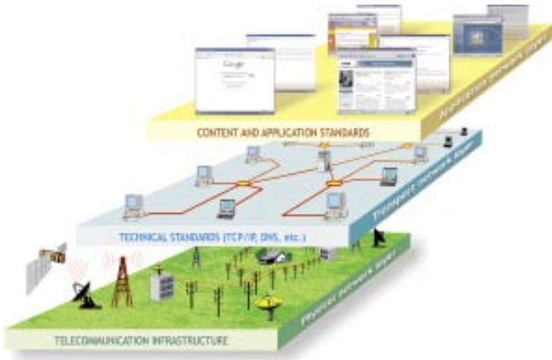
One of the Internet’s strengths is its layered architecture. The Internet Infrastructure layer remains independent of the telecommunications infrastructure (the layer below) and of the applications standards (the layer above).
